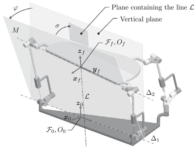
Fig. 2. Ideal form of architecture solution presented with 2-UPU and 1-SPU legs.
