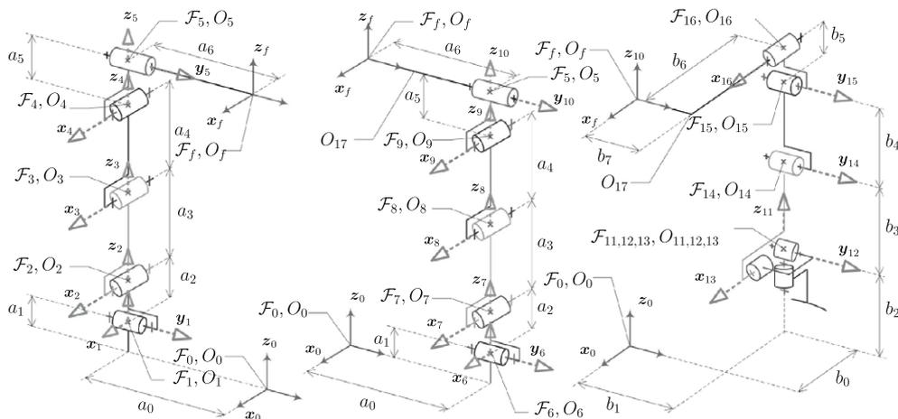
**Fig. A.1.** Screw axis definition for chains C1, C2 and C3 sketched in reference position.
