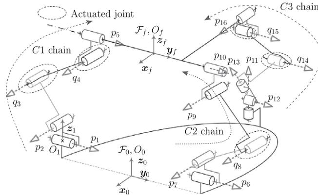
Fig. 4. Kinematic structure of the assembled mechanism.
