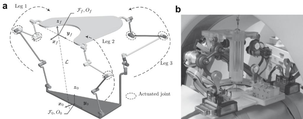
Fig. 3. Solid model and prototype of the mechanism in the CT-scanner ring.
