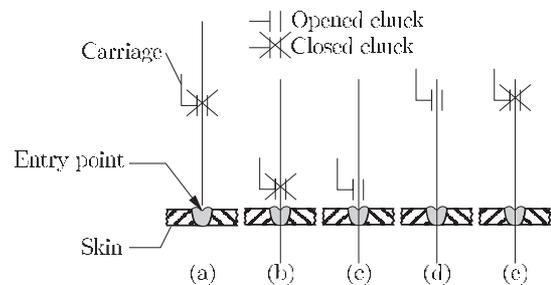
Fig. 4. Insertion cycle carried out with a chuck.
