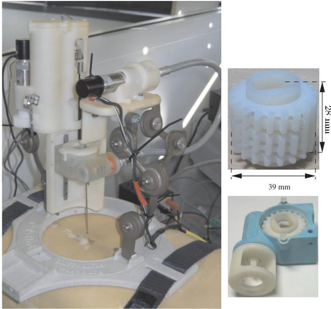
Fig. 9. Fabricated prototype of the insertion device, the chuck and the carriage.
