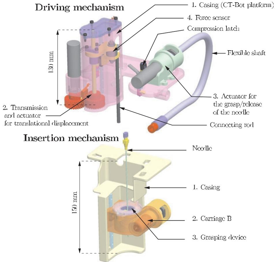
Fig. 5. Exploded view of the needle insertion driver.
