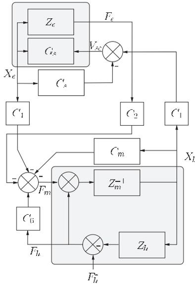
Fig. 14. Three-channel bilateral control scheme used in the experiments.
