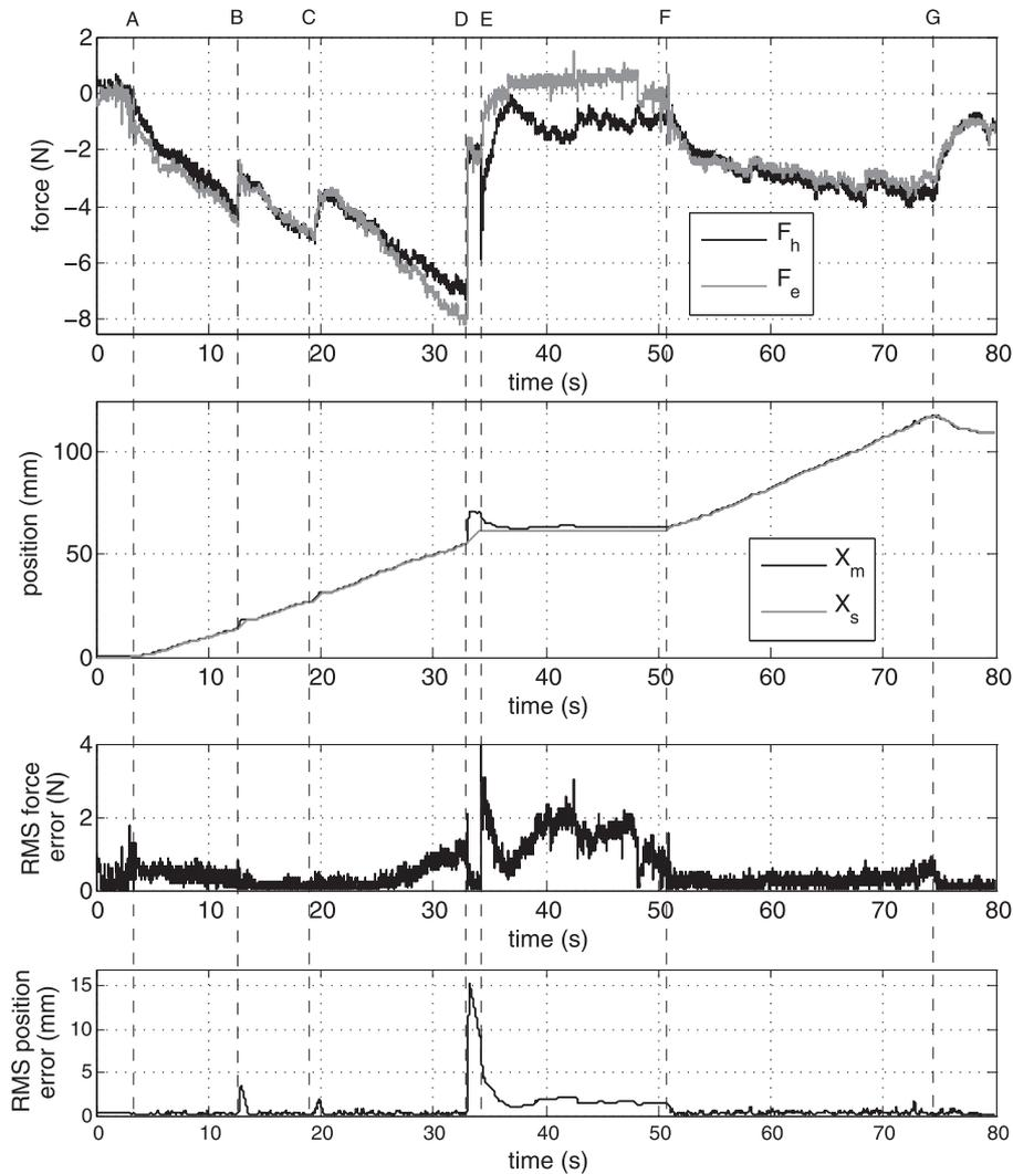
Fig. 18. Sequential needle insertion experiment. From top to bottom: force and position tracking between the master and the slave robots; RMS force and position tracking errors.
