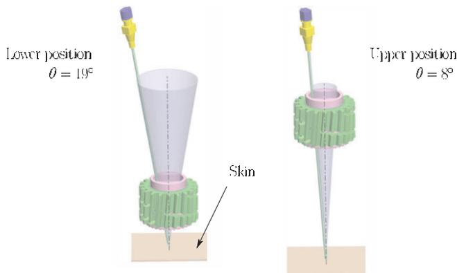
Fig. 12. Free motion of the needle for two carriage positions.
