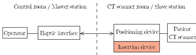
Fig. 2. General layout for a teleoperated percutaneous procedures.
