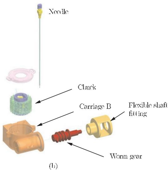
Fig. 7. Exploded view of the carriage B.
