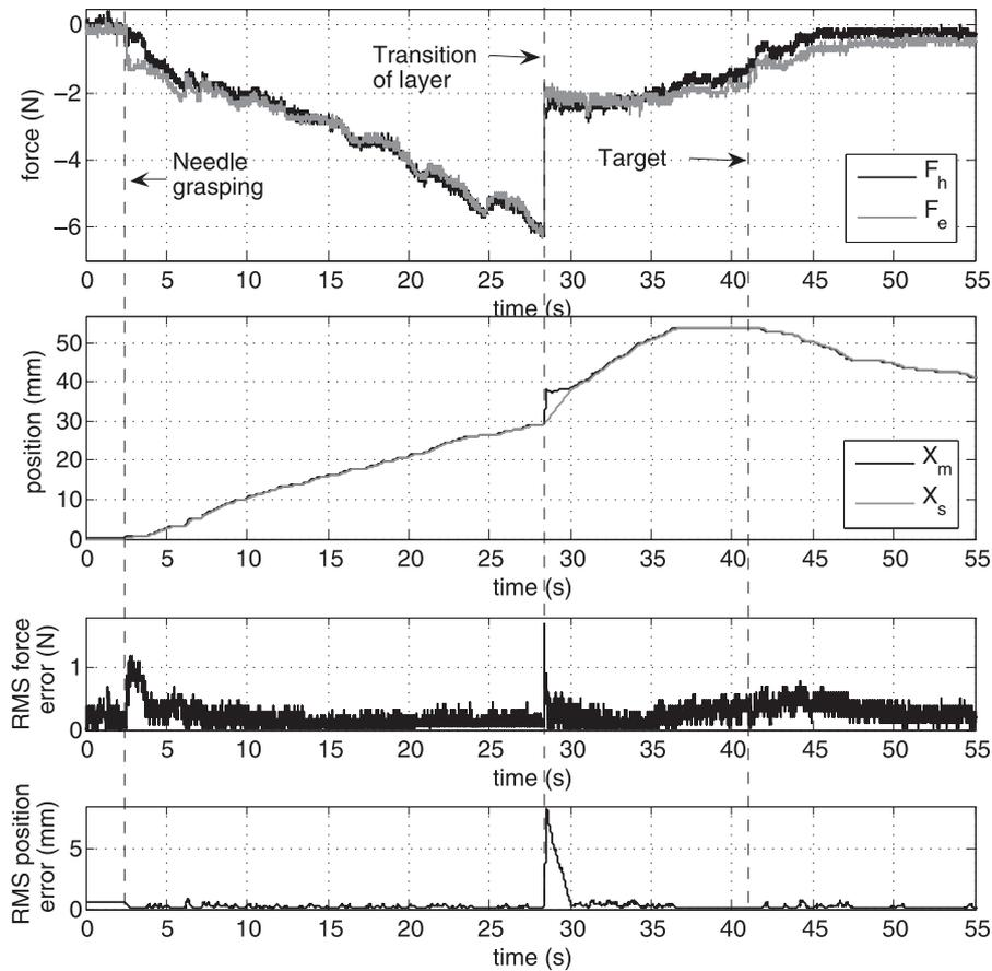
Fig. 17. Continuous needle insertion experiment. From top to bottom: force and position tracking for the master and the slave robots; RMS force and position tracking errors.
