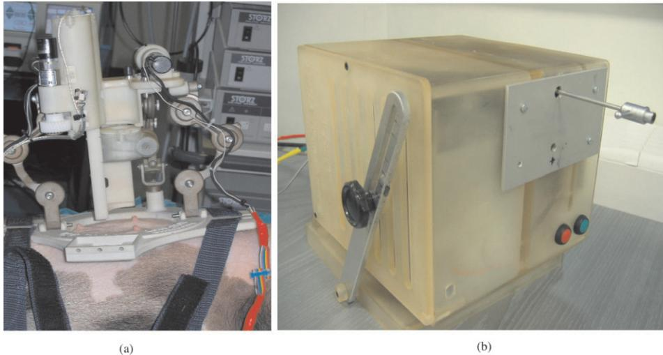
Fig. 13. Experimental setup: (a) needle insertion device, the slave manipulator mounted on an anesthetized swine; (b) CT-Master, the master manipulator.
