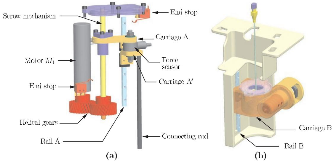
Fig. 6. Detailed views of (a) the driving mechanism and (b) the insertion mechanism.
