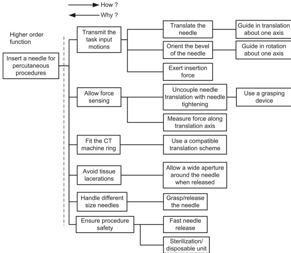
Fig. 3. Functional diagram of the needle insertion device.
