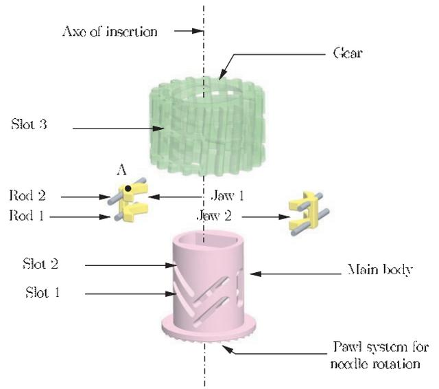
Fig. 8. Exploded view of the chuck.
