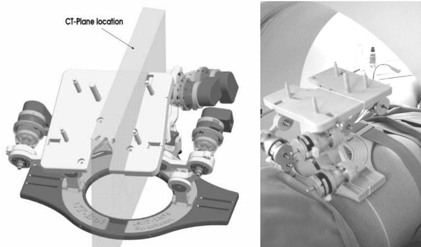
Fig. 1. The CAD model and the prototype under tests.
