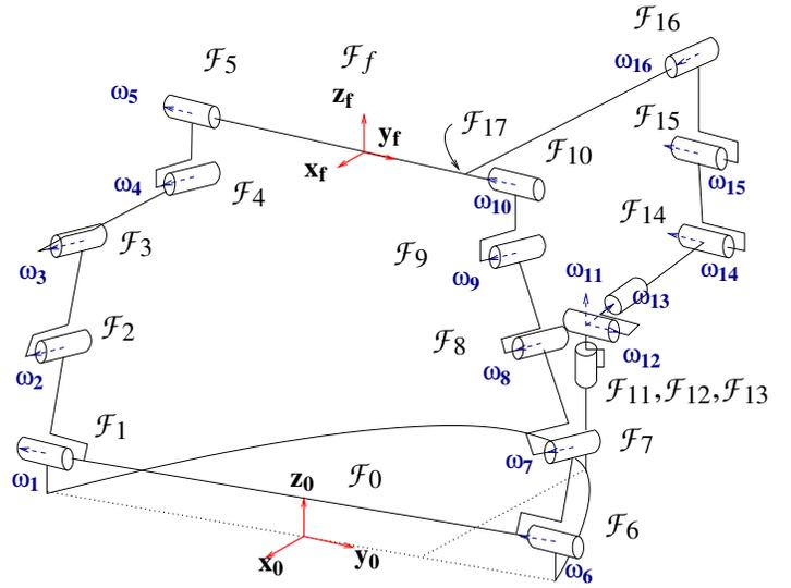
Figure 3. KINEMATIC MODEL OF THE ROBOT
