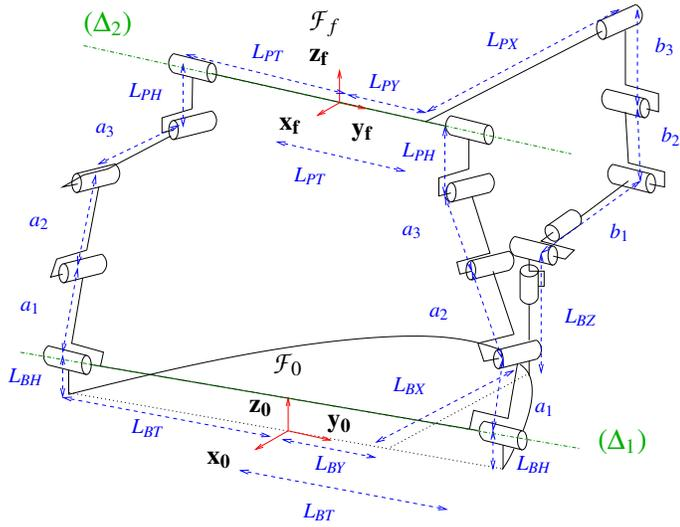
Figure 2. FUNCTIONAL SCHEMATIC OF THE ROBOT
