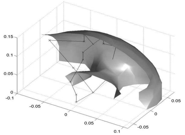
Figure 6. SIMPLIFIED WORKSPACE OF THE ROBOT
