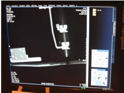
Fig 5. CT-image of the fiducials together with the needle, before the positioning.
