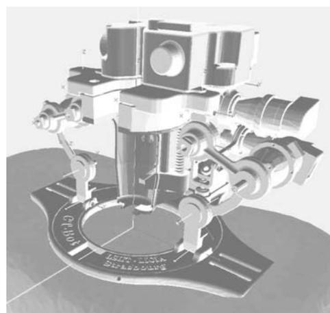
*Fig. 1: Computer Aided Design (CAD) model of the CT-Bot.*
