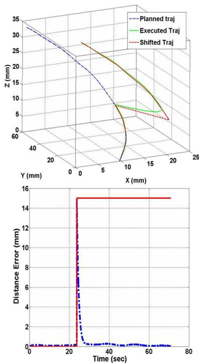
Fig. 5. Head tracking example. Planned trajectory (dashed-dot line in blue), same trajectory with a shift due to a head movement (dashed line in red) and coil trajectory obtained with the motion compensation module (solid line in green). Below: distance error.
