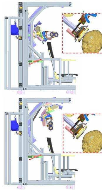
Fig. 2. Robot configuration before and after power failure. In dotted squares, the coil movement is represented with respect to the head.
