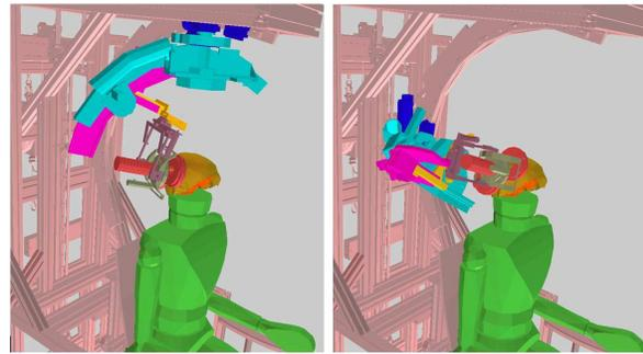
Fig. 4. Two robot configurations obtained during the motion execution. These configurations are far away from each other due to a joint limit avoidance made possible thanks to the motion planning algorithm.
