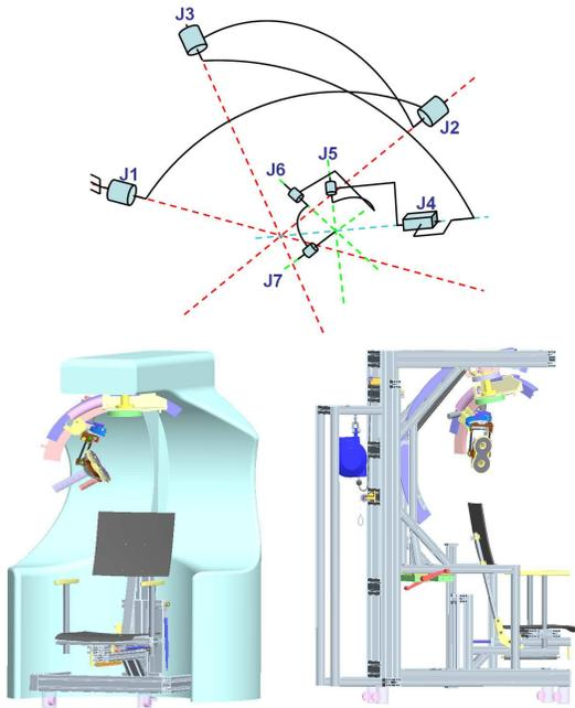
Fig. 1. The kinematics scheme and the CAD model of the robot.
