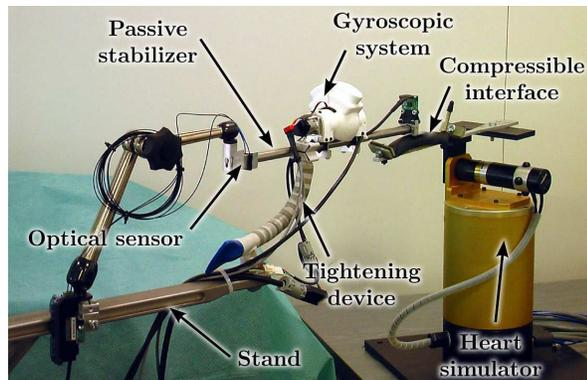
Fig. 4. Experimental setup overview.
