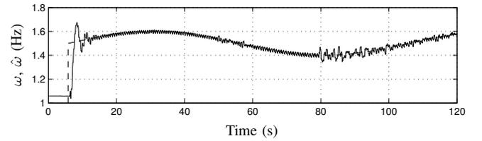
Fig. 8. Frequency estimation results. In dashed line the real perturbation frequency  $\omega$  and in plain line its estimate  $\hat{\omega}$ . The frequency estimation parameters are the following:  $\xi_e = 0.1$ ,  $k_e = 1000$  and  $g_e = 1000$ .
