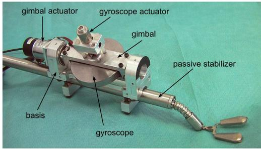
Fig. 3. System overview, here mounted on a passive stabilizer from Medtronic designed for minimally invasive beating heart surgery. The tip with the two fingers is inserted into the body while the gyroscopic system remains outside.
