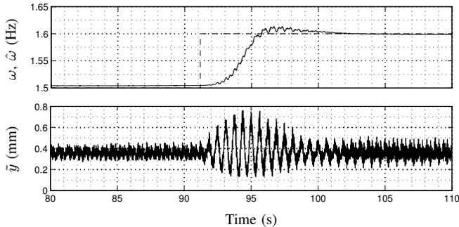
Fig. 9. Adaptive algorithm with frequency estimation results. On top the real perturbation frequency  $\omega$  is in dashed line and the estimate  $\hat{\omega}$  in plain line. On bottom the stabilizer displacement measurement  $\hat{y}$ .
