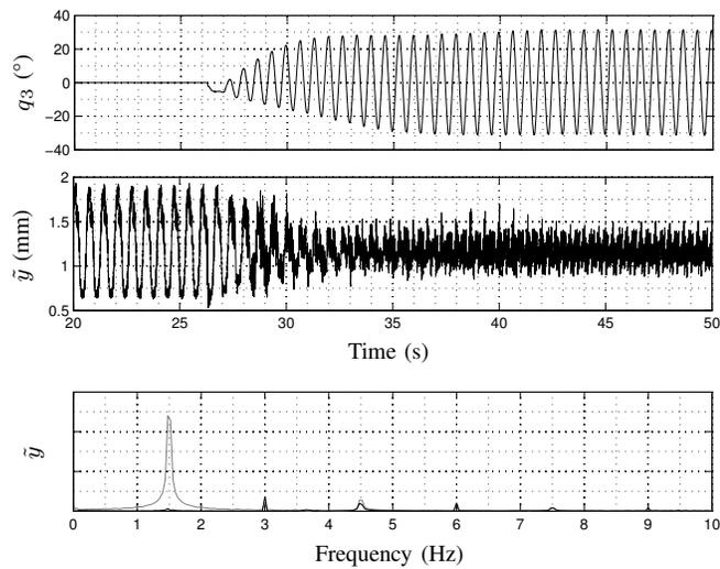
Fig. 7. Adaptive algorithm results with known cardiac frequency  $\omega = 1.5$  Hz and  $g = 0.5$ . On top the gimbal angular displacement  $q_3$  and in the middle the stabilizer measured displacement  $\tilde{y}$ . On bottom the comparison of the frequencial decomposition of the measured displacement  $\tilde{y}$ , with compensation ( $t > 35$  s) in black and without ( $t < 25$  s) in gray.
