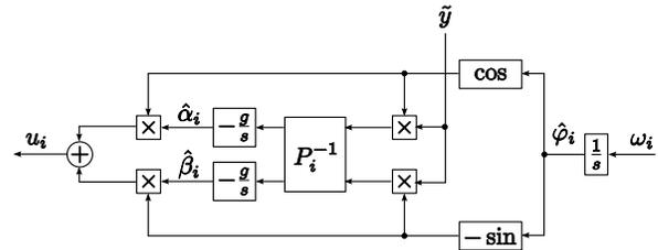
Fig. 6. Adaptive compensation control scheme for one harmonic.
