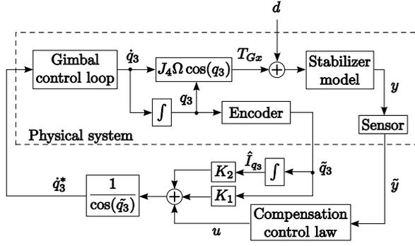
Fig. 5. Overall control scheme.
