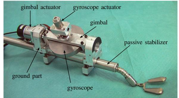
Fig. 2. System overview, here mounted on a passive stabilizer from Medtronic.
