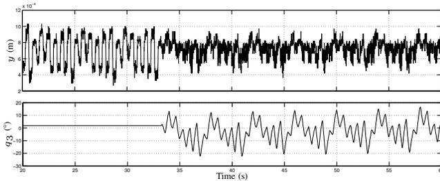
(a) Compensation results for position  $y$  and gimbal angle  $q_3$ . Compensation is activated at  $t = 33$  s.
