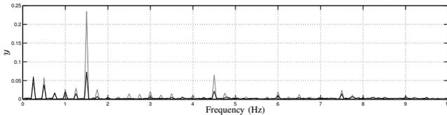
(b) Comparison of unstabilized (gray) and stabilized (black) results in frequency domains. Data are extracted respectively for  $t = 10$  to  $30$  s and  $t = 40$  to  $60$  s.
