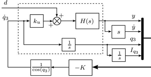
Fig. 3. Structure of the system controlled with static state feedback  $K = [k_1 \ k_2 \ k_3 \ k_4]$ . Dashed line delimits the gyrosopic system itself.
